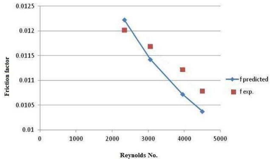
**Fig. 3: Comparison of experimental values of friction factor with the values predicted by Blasius's equation for smooth collector**
