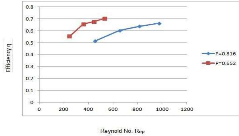
Fig. 8: Effect of Reynolds number & porosity on efficiency
