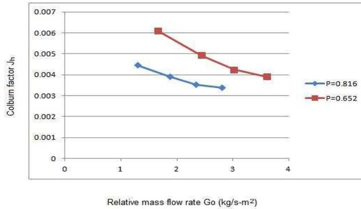
Fig. 10: Effect of Colburn factor & porosity on Relative mass flow rate
