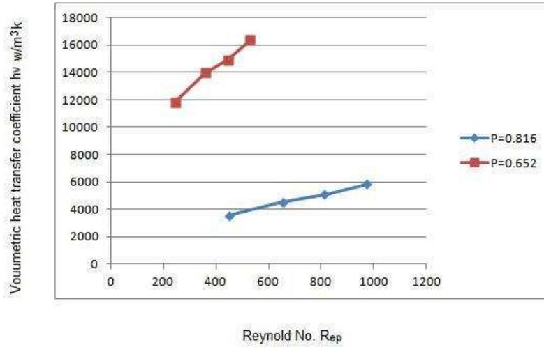
Fig. 4: Effect of Reynolds number & porosity on volumetric heat transfer coefficient
