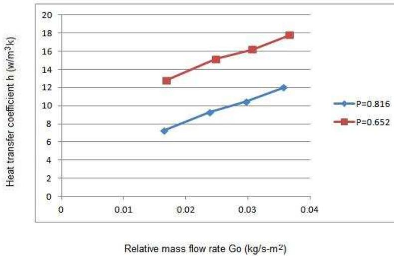
Fig. 5: Effect of relative mass flow rate and porosity on heat transfer coefficient
