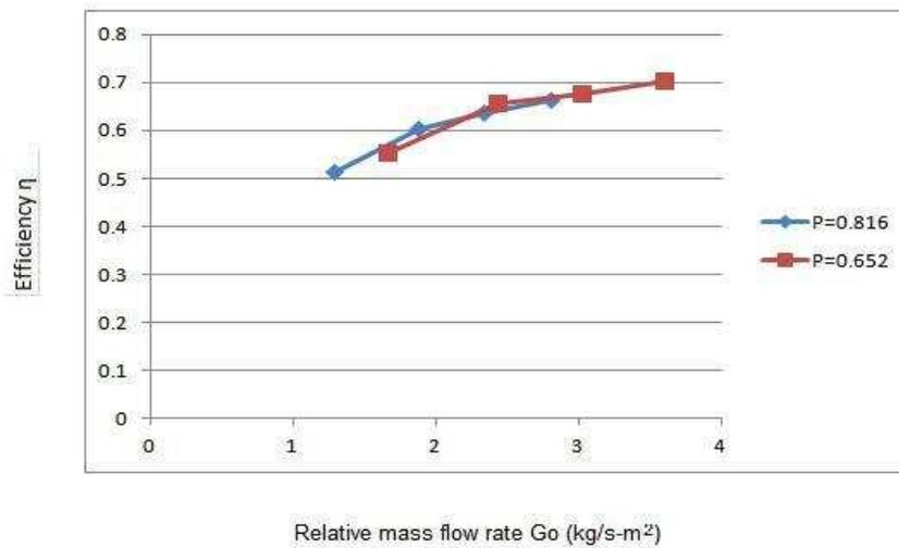
Fig. 7: Effect of Relative mass flow rate & porosity on efficiency
