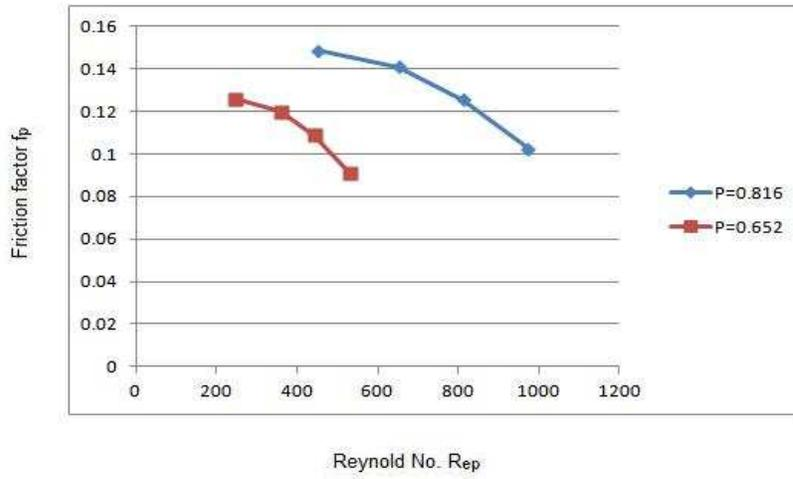
Fig. 6: Effect of Reynolds number & porosity on friction factor
